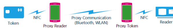
Figure 5: representation of a relay attack using a contactless smartcard, 2 NFC equipped phones and a reader terminal.
