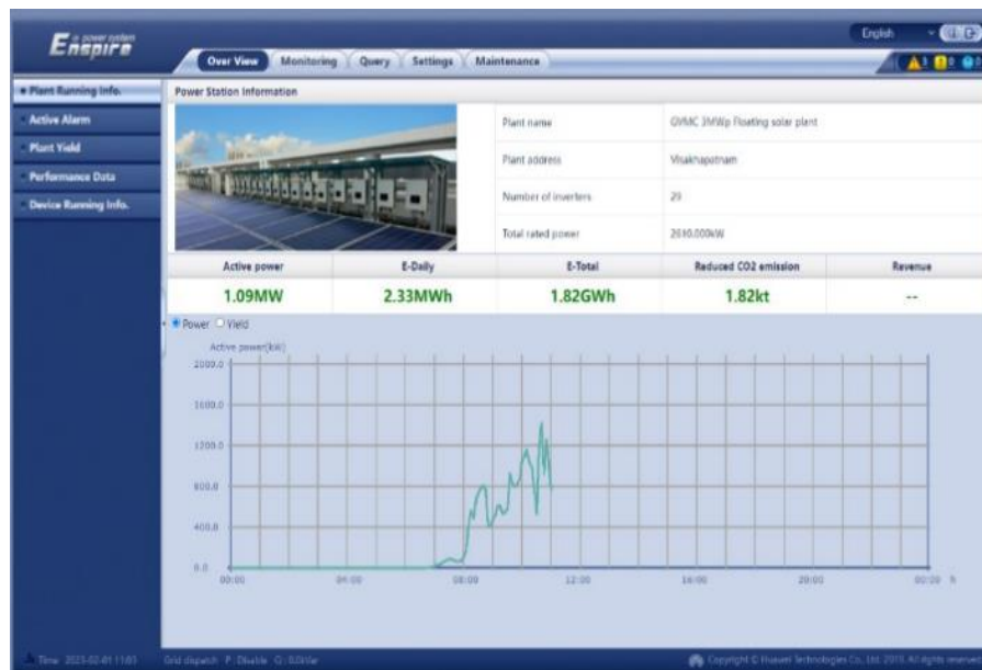
Fig.11 : SCADA monitoring system performance captured on 31.01.2023
