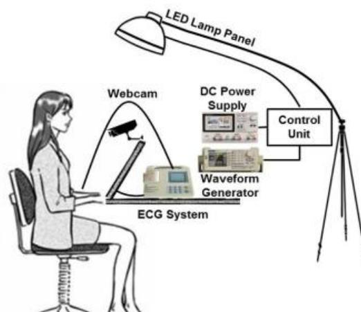
Fig. 3. Ideal Experimental Setup for HR Detection [5].
