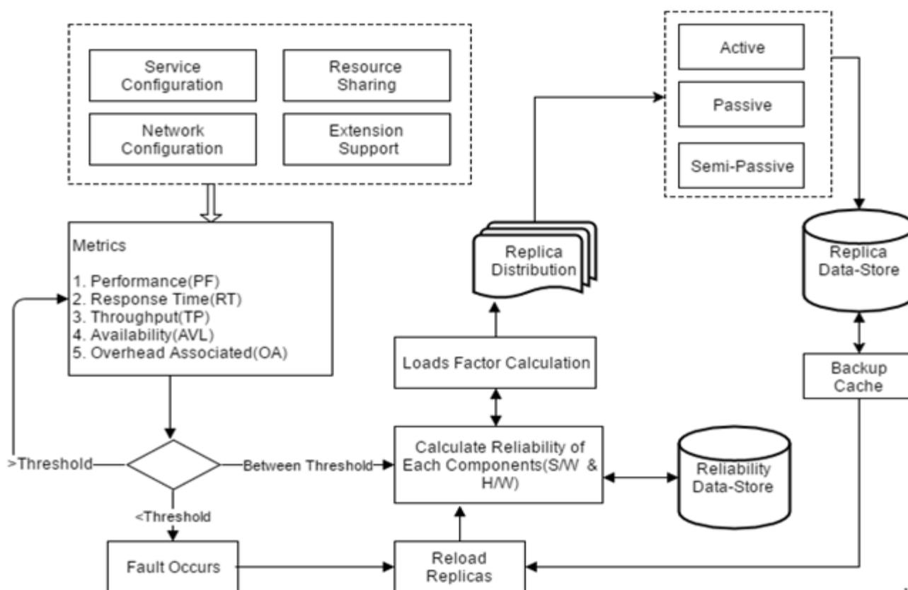
Figure 1: Design Architecture of Proposed RAI-DD Fault Tolerance Model.
