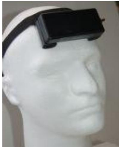
Fig.5: Example of Wireless EEG
