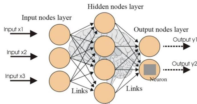
Fig 1: Structure of an artificial neural network
