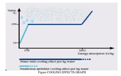
That's why high pressure water mist cools efficiently per liter of water up to seven times better than can be obtained with one litre of water used in a traditional sprinker system.
