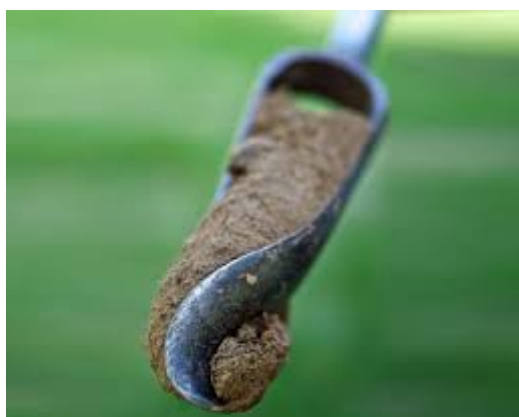
Fig. 6 : Taking soil samples using auger equipment
