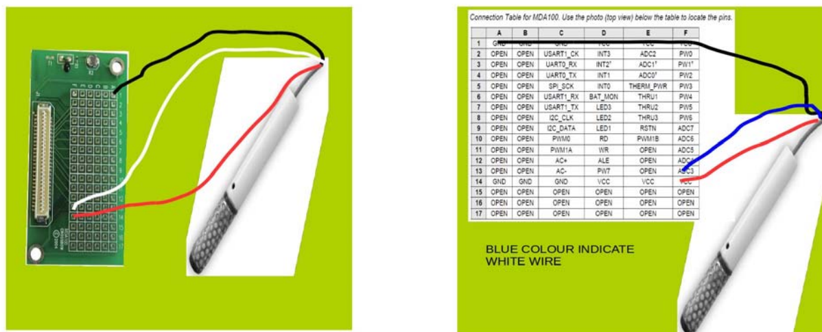
Fig 5. Watermark Soil Moisture Meter with MDA 100 Sensor board (real and with Pin diagram)
