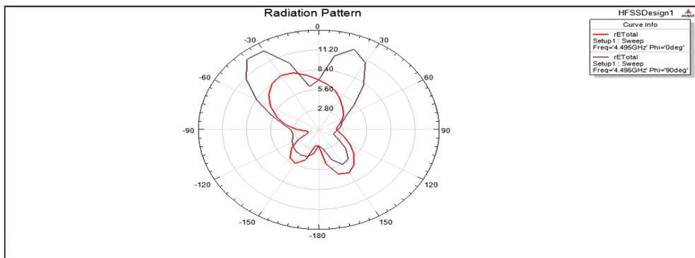
Fig. 5 Radiation Pattern at 4.5 Ghz
