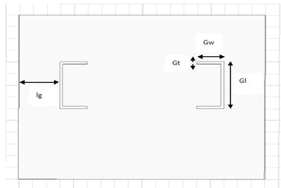
Fig. 2. Back view of antenna showing the ground slots
