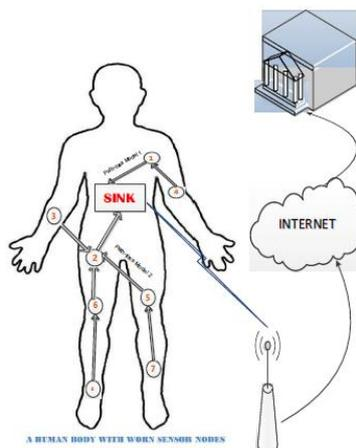
Figure 1: Schematic Diagram for LAEEBA Protocol
