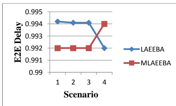
Figure 4: Comparison of E2E Delay between LAEEBA and MLAEEBA
