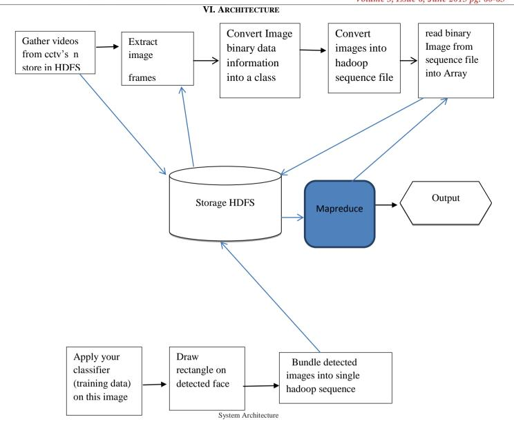
This system provides the application interface for users. The system incorporates two phases -1) Upload the images and 2) Search the image from the database. Both modules are deployed on Hadoop cluster. For uploading phase, the data is inputted for storage of HDFS and Query Image is searched from the database.
