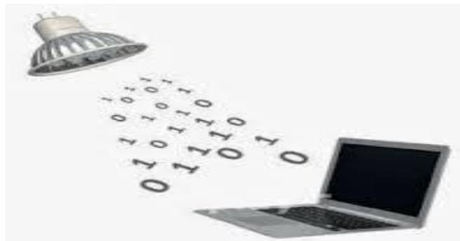
On one end all the data on the internet will be streamed to a lamp driver when the LED is turned on the microchip converts the digital data in form of light sensitive device (photo detector) receives the signal and converts it back into original data. This method of using rapid pulses of light to transmit information wirelessly is technically referred as Visible Light Communication
