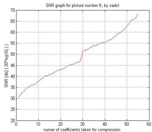
Figure 8: SNR graph using SA-DCT
