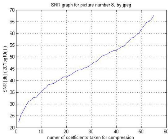
Figure 7: SNR graph using JPEG
