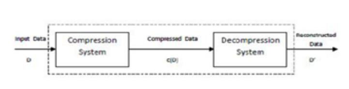
Figure 1: Block Diagram of CODEC
