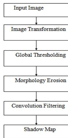
Fig. 2: New algorithm for the shadow detection
