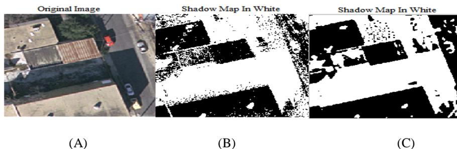
Fig. 3: (a) Original image. (b) Shadow detection by Tsai's method. (c) Shadow detection by new algorithm.
