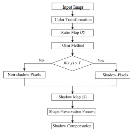
Fig. 1: Tsai algorithm
