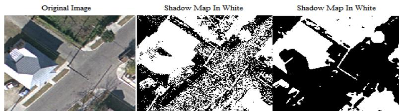
Fig. 4: (a) Original image. (b) Shadow detection by Tsai's method. (c) Shadow detection by new algorithm
