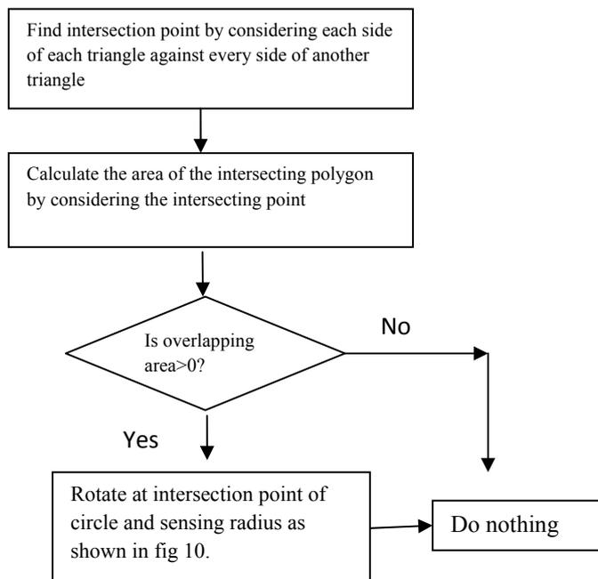
Fig 9: Flow Chart for checking intersection point
