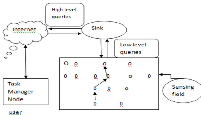
Fig 1: Architecture of sensor network
