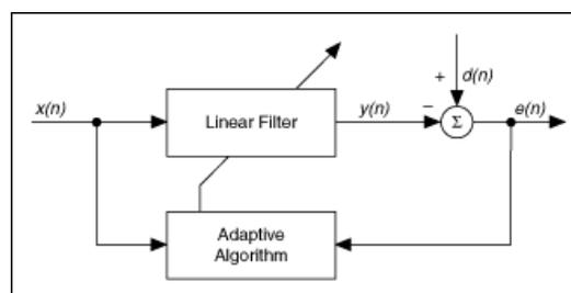
Fig: Block diagram of adaptive filter
