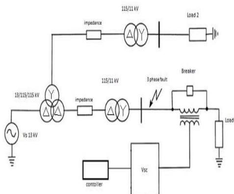
Figure-6: Single line diagram of test system of DVR
