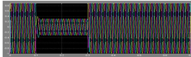
Figure-12: 3phase voltage at load point without DVR at three phases to ground fault
