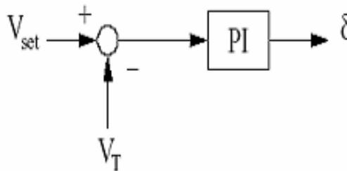
Figure-3: Indirect PI controller
