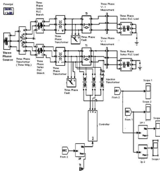
Figure-7: Simulink model of DVR
