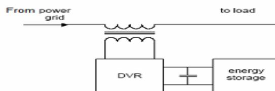
FIGURE-1: EXAMPLE OF A STANDARD CONFIGURATION FOR A DVR.
