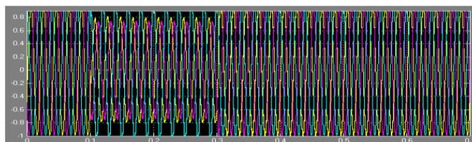
Figure-15: 3phase voltage at load point with DVR at two phases line to line fault
