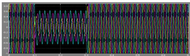
Figure-10: 3phase voltage at load point without DVR at double line to ground fault
