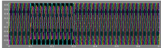
Figure-11: 3phase voltage at load point with DVR at double line to ground fault
