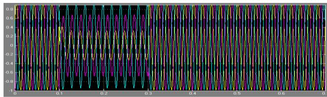
Figure-14: 3phase voltage at load point without DVR at two phases line to line fault
