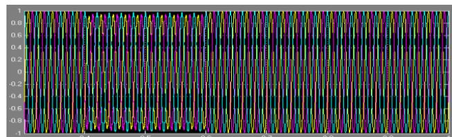
Figure-9: 3phase voltage at load point with DVR at single line to ground fault
