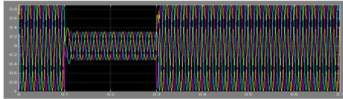
Figure-14: 3phase voltage at load point without DVR at three phases line to line fault
