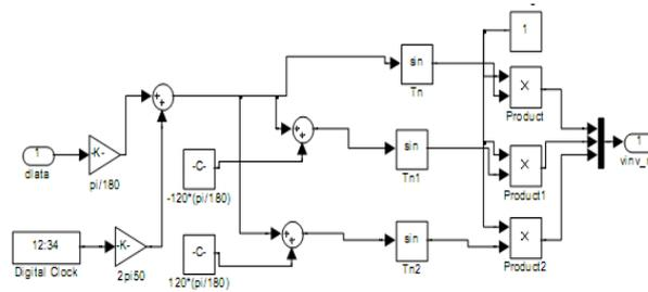
Figure-4: Phase modulation of control angle  $\delta$
