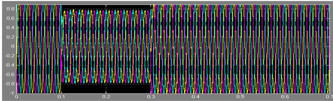
Figure-15: 3phase voltage at load point without DVR at three phases line to line fault
