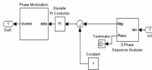
Figure-5: Simulink model of controller of DVR
