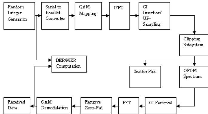
Fig.1 OFDM transceiver model for clipping
