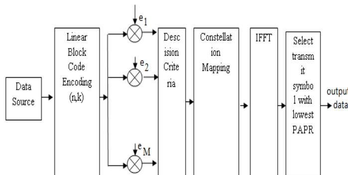
Fig 3. Block diagram of MSLM reduction technique.
