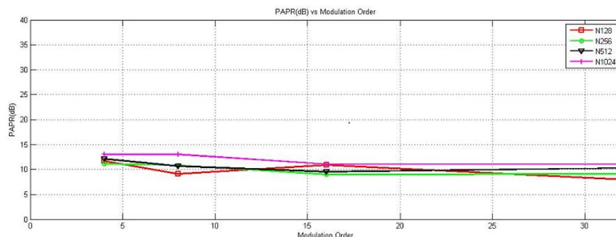
Fig. 4 PAPR Vs modulation order for different no. of subcarriers
