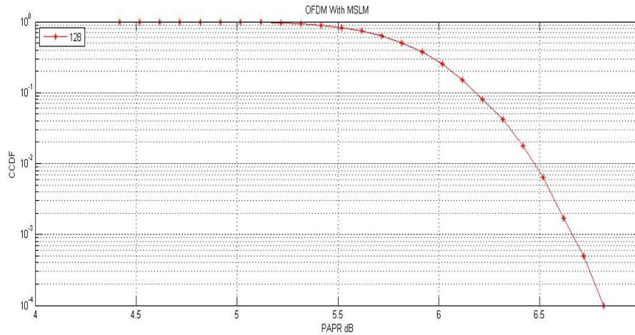
Fig. 7 PAPR Reduction for MSLM where N = 128.
