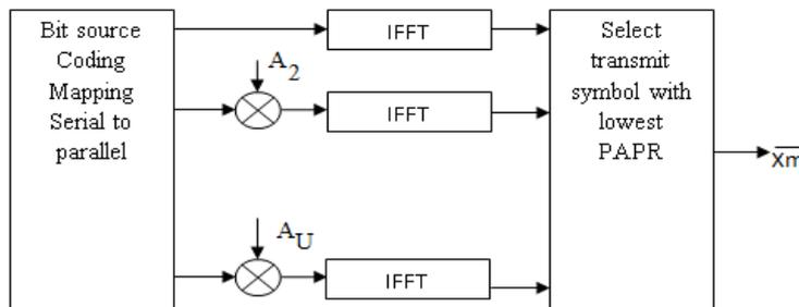
Fig. 2 Block diagram of SLM reduction technique.
