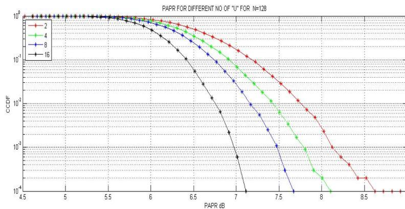
Fig. 6 PAPR with variation of no. of U for SLM where N = 128
