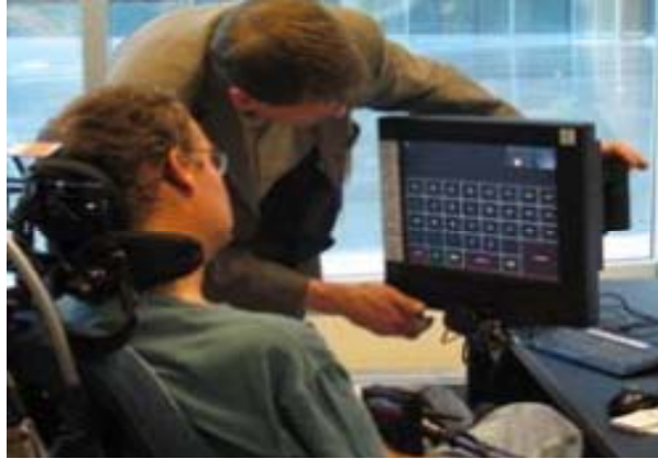
Gaze detection pointing system for people with disabilities (taken from www.adamfulton.co.uk )
