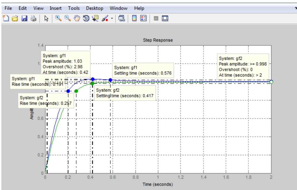
Fig 3. Step response for two controlled system
