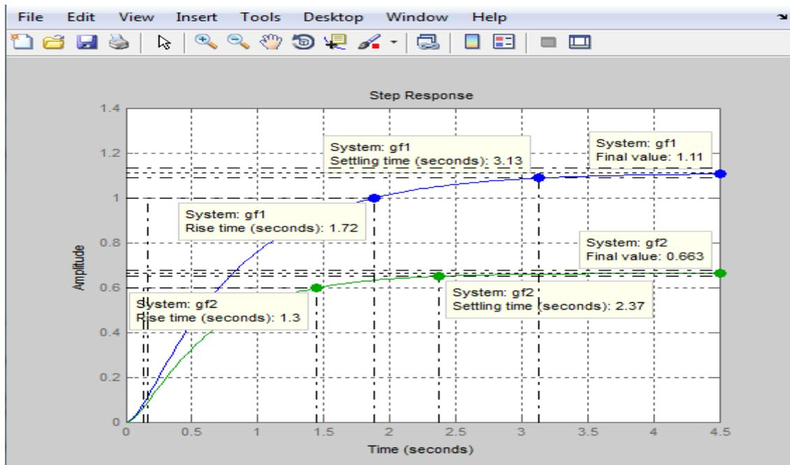
Fig 2. Step response for two transfer function  $gf_1$  &  $gf_2$
