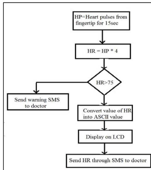
Fig. 7 Flow chart of Heart Rate monitor
