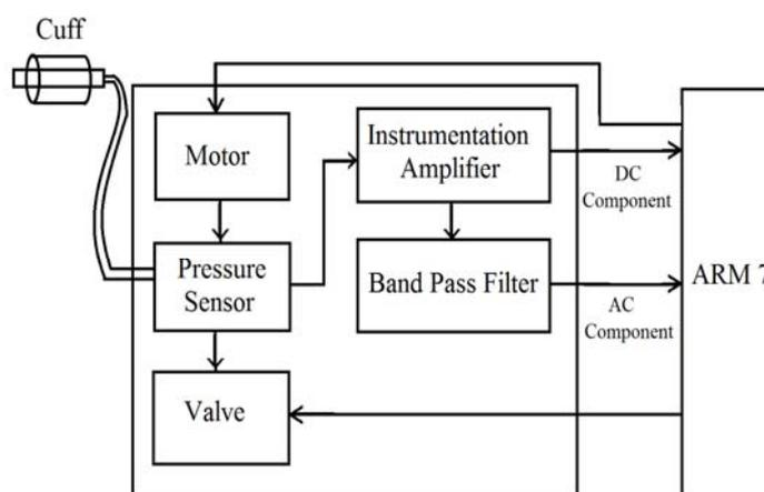
Fig. 2 Block diagram of portable digital BP monitor.
