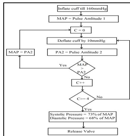
Fig. 6 Flow chart of Blood pressure monitoring
