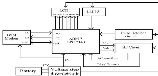
Fig. 1 Block diagram of GSM based telealert system
