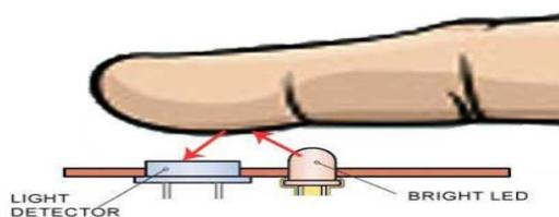
Fig. 3 Working operation to measure Heart rate.
