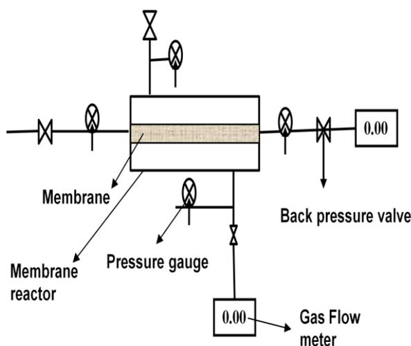
Fig 3: Gas permeation experimental set up for Hydrogen Production and Purification through a Membrane inside a membrane reactor
