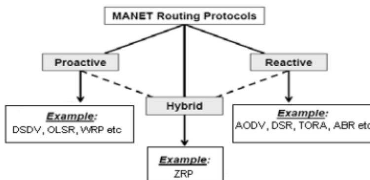
Figure2. Classification of MANET routing protocols
