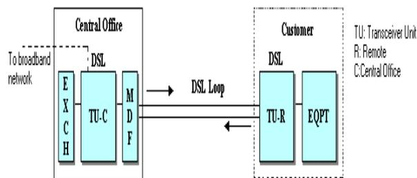
Fig-2 General Model of DSL systems
