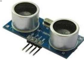
Figure 4. Ultrasonic sensor
