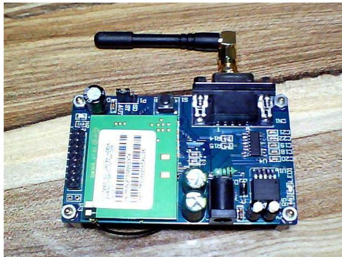
Figure 5. GSM Modem
