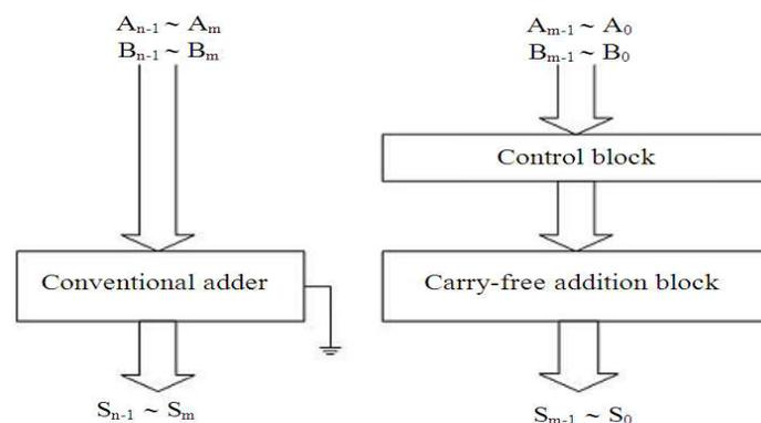
Fig.1 Logic Diagram of ETA Adder
