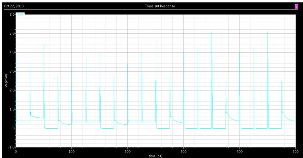
Fig. 67 Power waveform of ETA Adder
