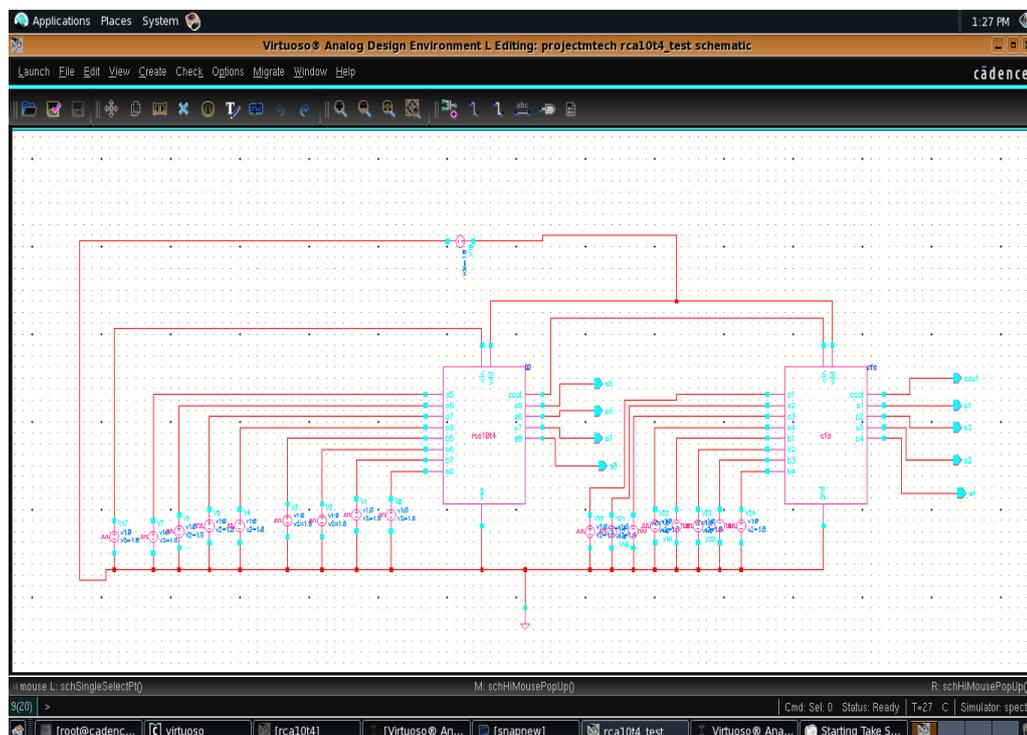
Fig.2 Block Diagram of ETA Adder
