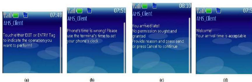
Fig. 3 (a) Touching a Tag (b) Phone’s time does not match Terminal’s time (c) User arrives late (d) Successful login after arrival
