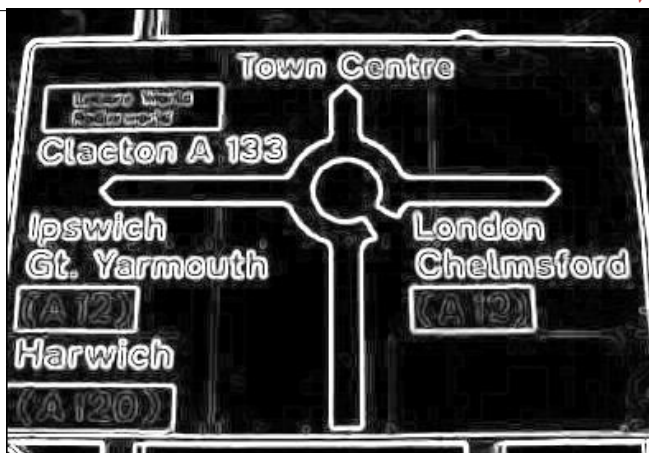
Fig.2: Edge detection by using Sobel operator
