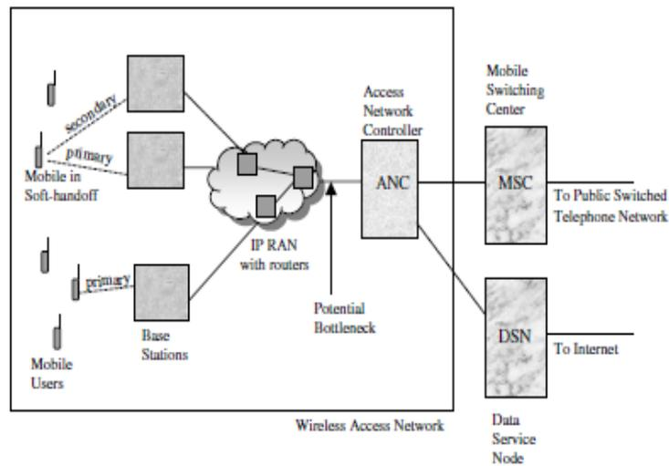
Fig. 1. CDMA Wireless Access Network with IP RAN
