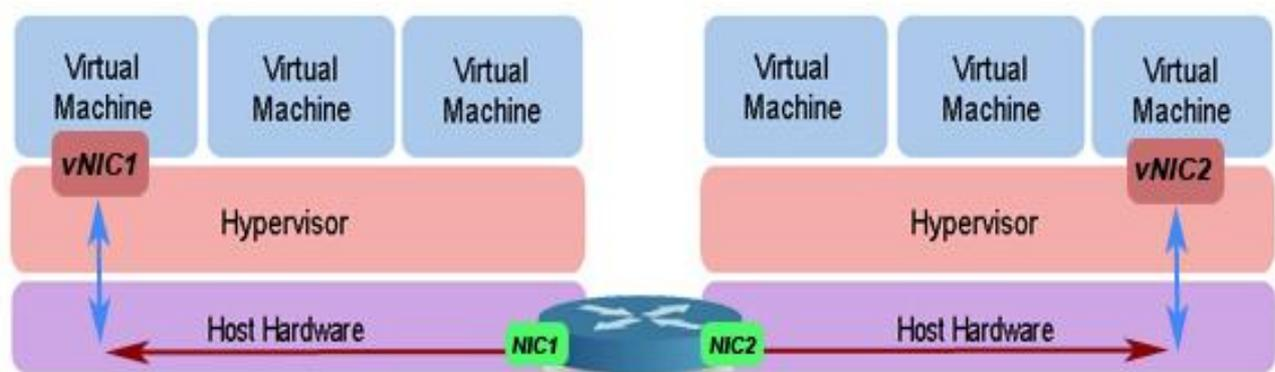
Figure 6: VMs communication on two physical hosts.
