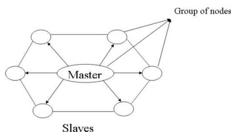
Fig 3 Schematic diagram of Coarse-Grained PGA
