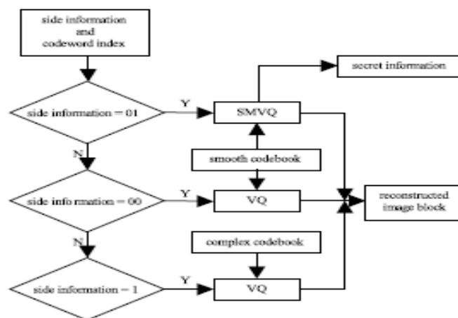
Fig.2. Block Diagram of Data extracting algorithm
