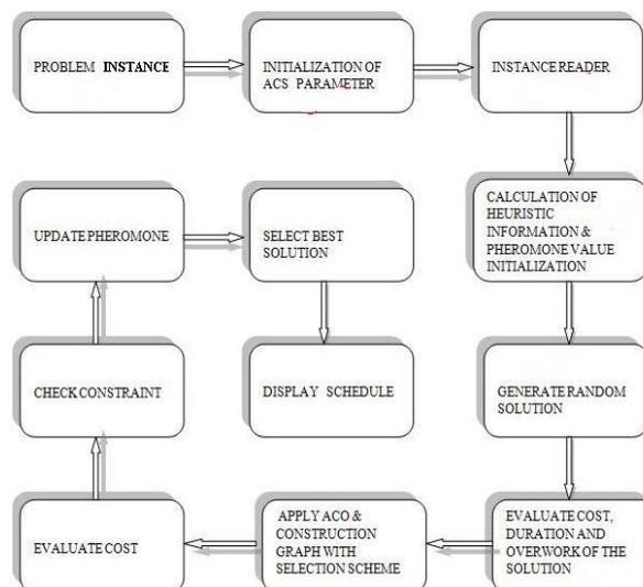
Fig 1. Block Diagram of SPP Problem
