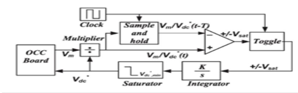
Fig. 3. Block diagram of the MPPT realization.
