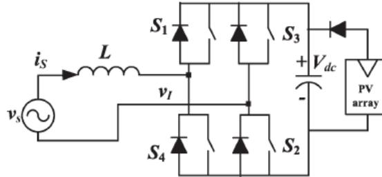
Fig. 1. Single-stage single-phase grid-connected PV system
