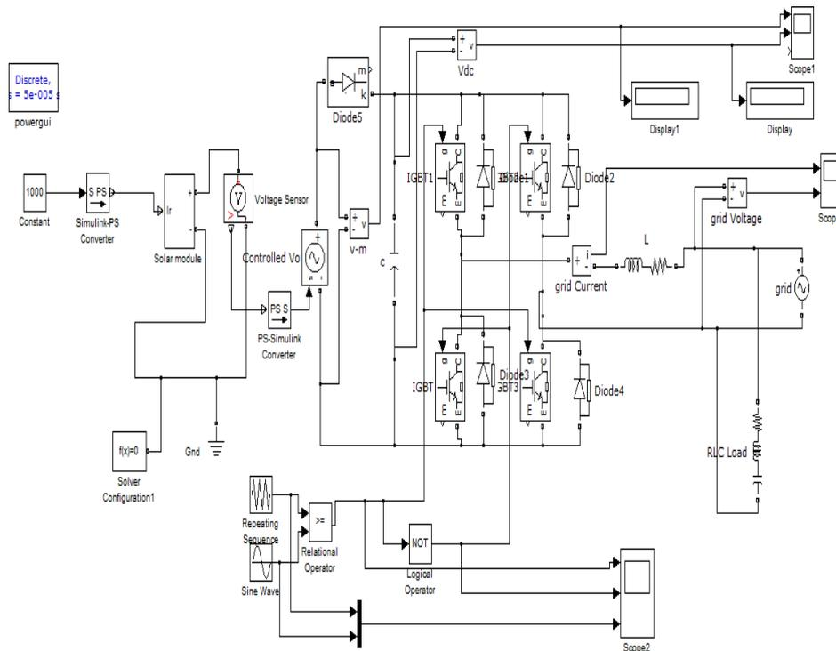
Fig. 4. Simulink model for grid connected inverter.
