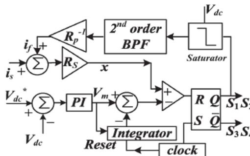
Fig. 2. Control block diagram of the proposed voltage-sensorless scheme
