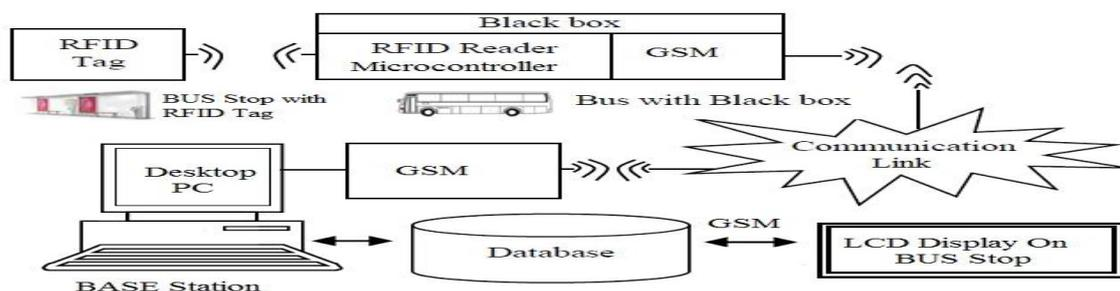
Figure 2: Architecture of Intelligent Bus Monitoring and Management System
