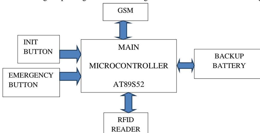
Figure 4: Block Diagram of In-BUS Module
