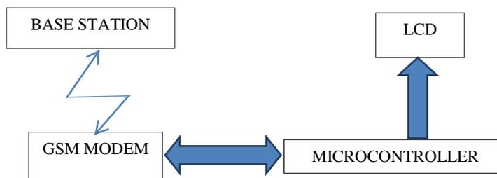
Figure 5: Block Diagram of BUS Stop Module
