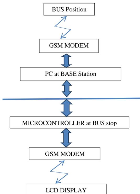
Figure 6: Block Diagram of BASE Station Module
