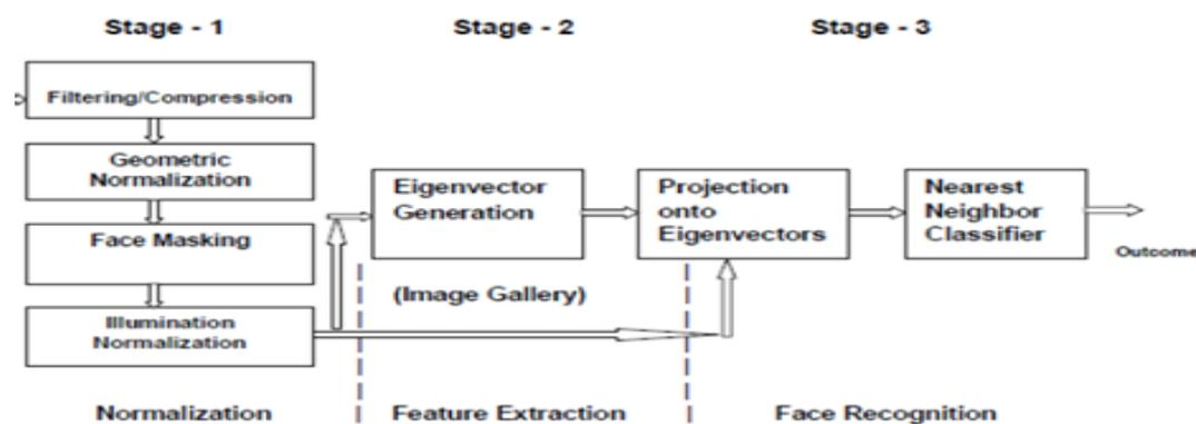
Figure 2 Block diagram for PCA based face recognition
