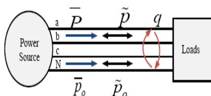
Fig. .2- Concept of different powers which are transferred and exchanged between power source and load [14]
