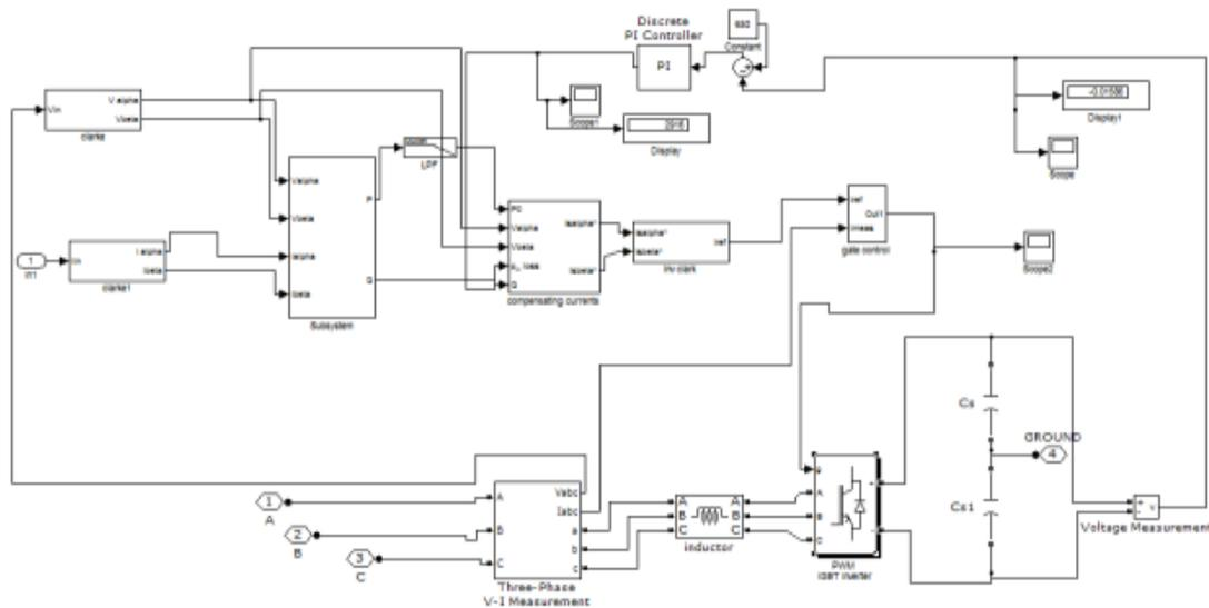
Fig.2- Subsystem of shunt active filter
