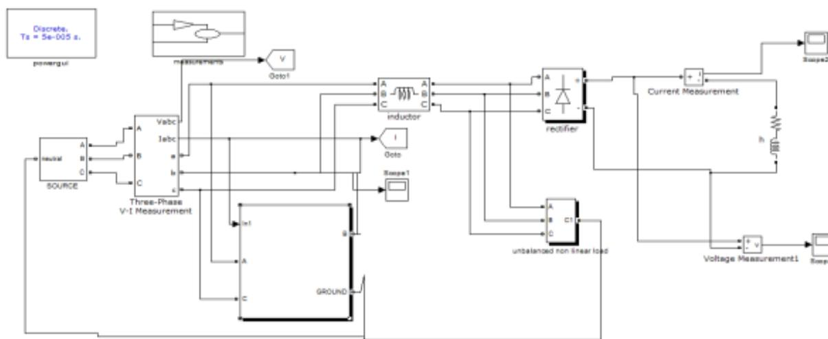
Fig.1- Complete diagram of Shunt Active Filter
