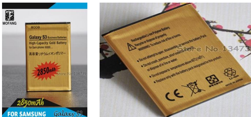
Fig.3 Front and Rear side of the Samsung S3 counterfeit battery
