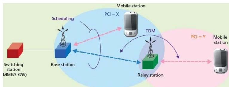
Fig. 1 Example of a Relay network.
