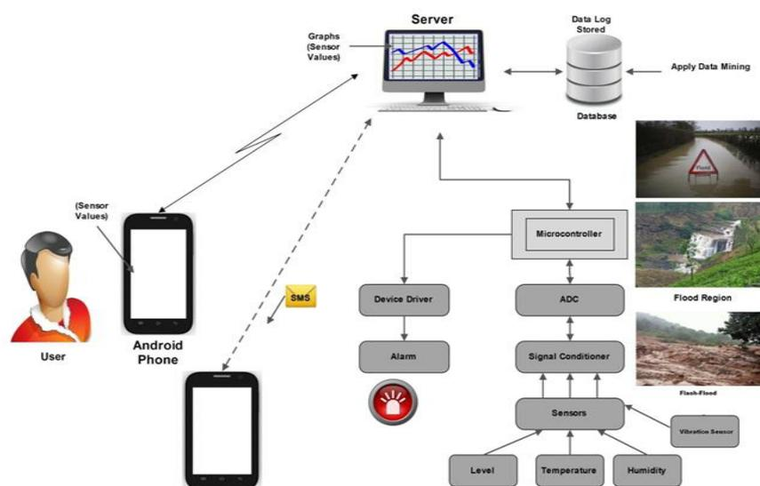
Fig.3 System Architecture
