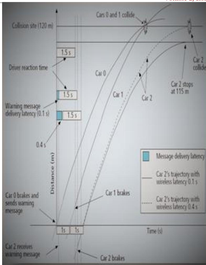
Fig.3.Cooperative collision avoidance (CCA) using vehicle-to-vehicle communications [3]
