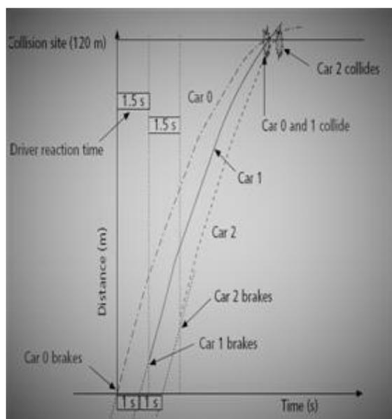
Fig.2b. Chain car collision when drivers react only on the tail light of the car ahead [3]
