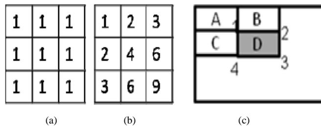
Fig. 3: (a) Input image (b) Integral image computation for input image (c) Calculation of the rectangular box from integral image.
