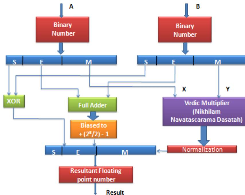
Fig. 3 Block Diagram of Universal Multiplier
