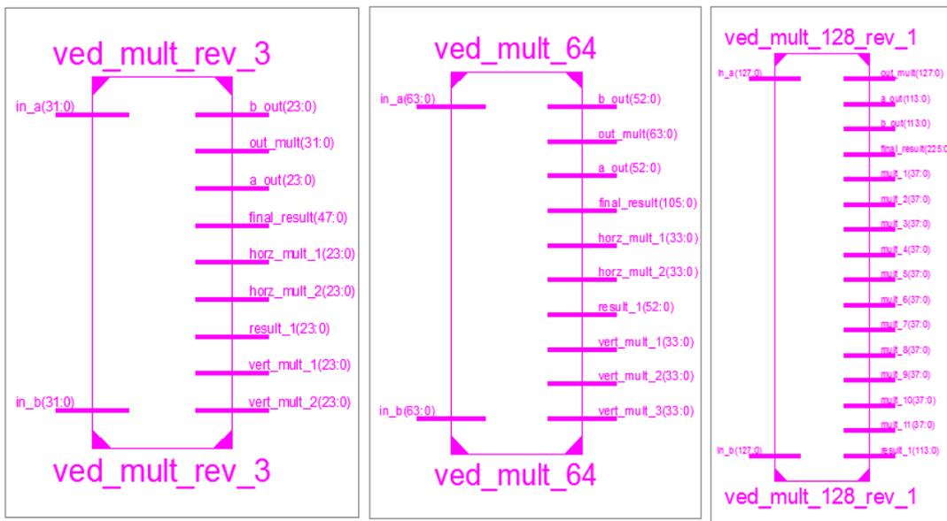
Fig. 6: RTL schematic for single, double and quadruple precision multipliers
