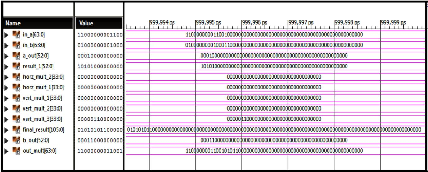
Fig. 5 : Test-bench waveform for 64-bit multiplier
