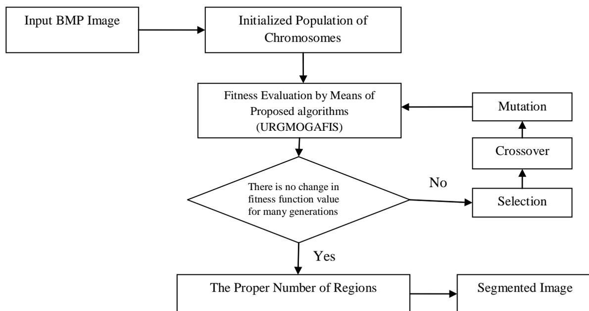
Fig -3 Schematic flow chart of segmentation
