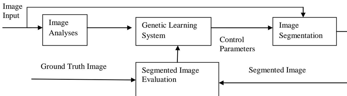
Fig-4 Block Diagram of Adaptive Image Segmentation
