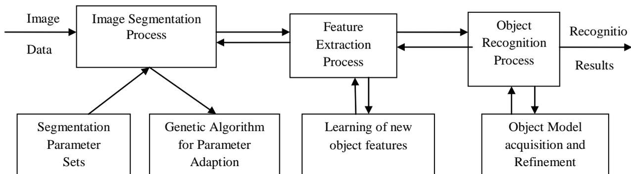
Figure -2 Conceptual design of the multi-level computer vision process
