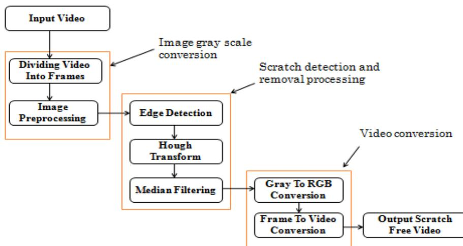
Fig. 3: block diagram for scratch detection and removal process
