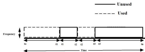
Fig. 3 Utilizing of Assigned Spectrum
