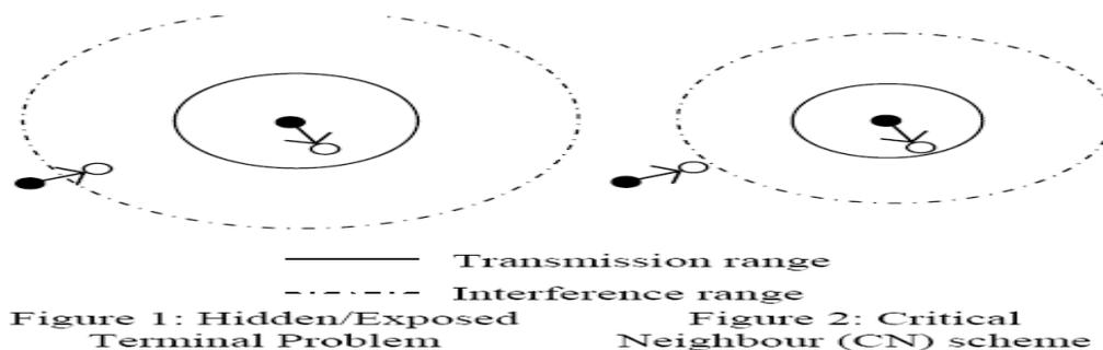
The Critical Neighbor scheme complements the RTS/CTS dialogue to reduce the collisions within the interference range. By reducing the transmission range of nodes such that they reach the minimum distance required to maintain connectivity with the neighboring nodes that are part of the active routes, unnecessary interference experienced by other neighboring nodes can be minimized.
