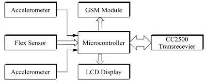
FIGURE1: FUCTIONAL BLOCK DIAGRAM
