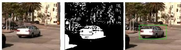
Fig 3.(a)original image (b) foreground image (c)moving object detection such as car.
