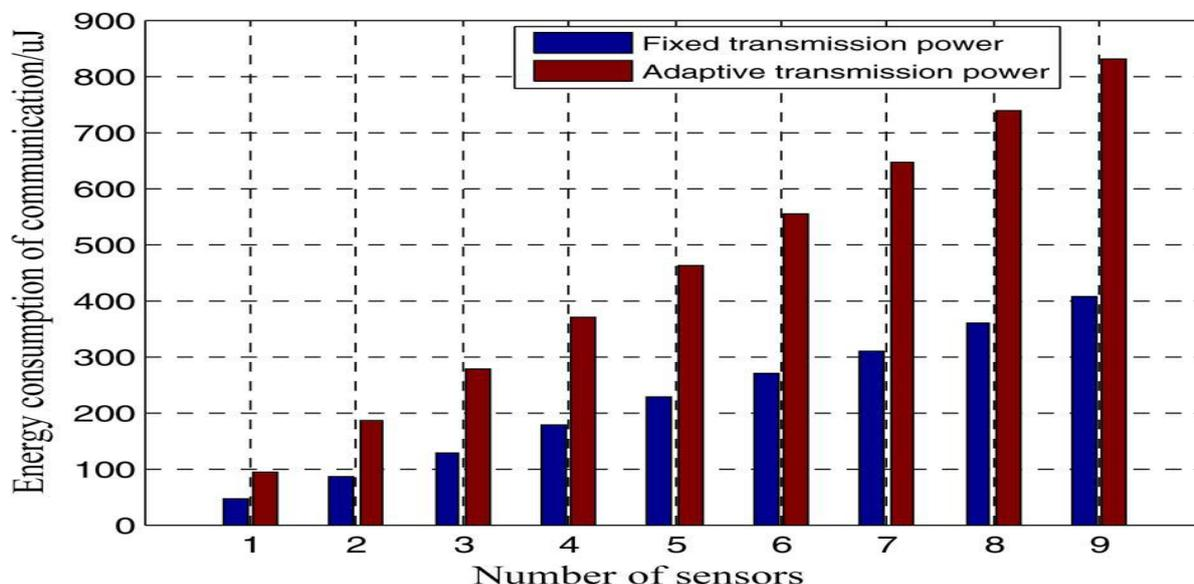
Fig 2. Communication energy consumption of the sensor network with different scales.
