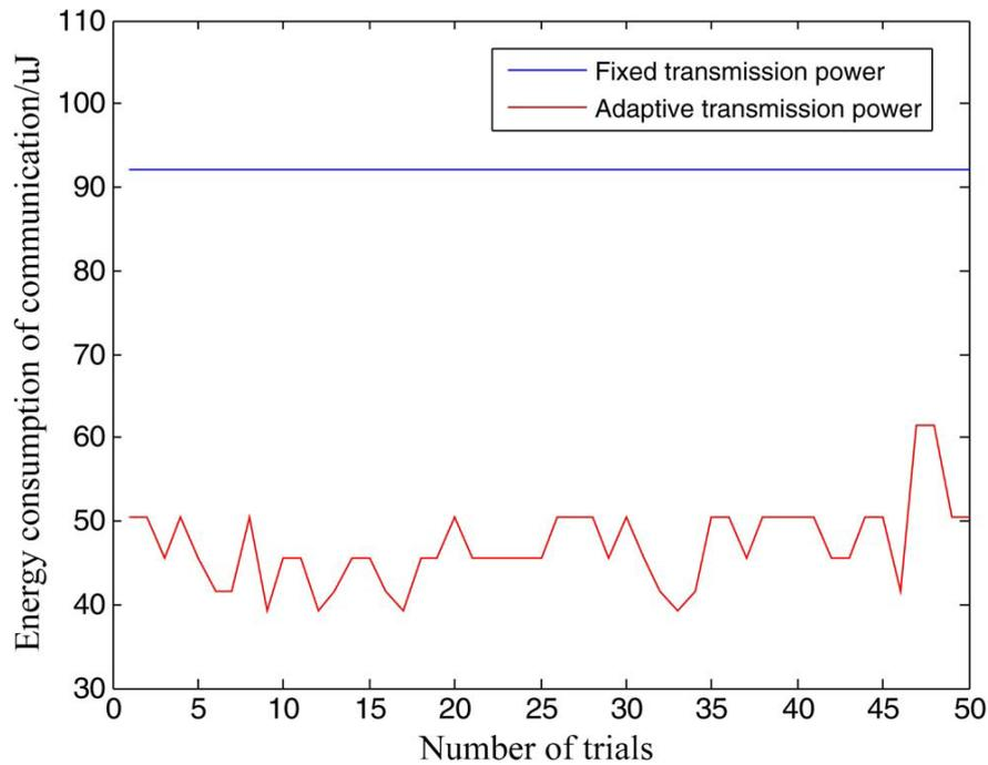
Fig. 3. Communication energy consumption under different transmission power settings.
